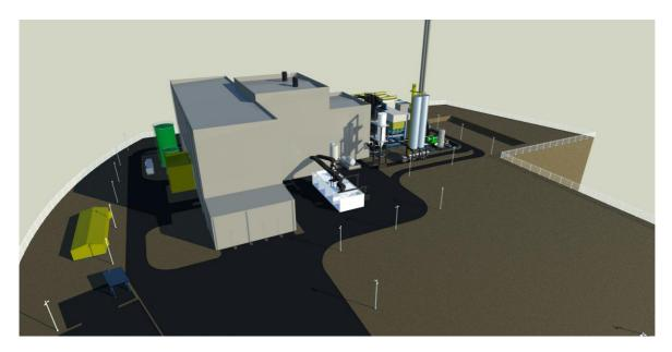
The Hooton Bio Power facility will be the fifth Energy from Waste (EfW) project delivered by leading renewable energy developer CoGen and will be the first non-subsidised merchant gasification facility. It is the first time the UK market will realise a gasification plant of this size, based on fluidised bed technology provided by Japanese Kobelco Eco Solution.
